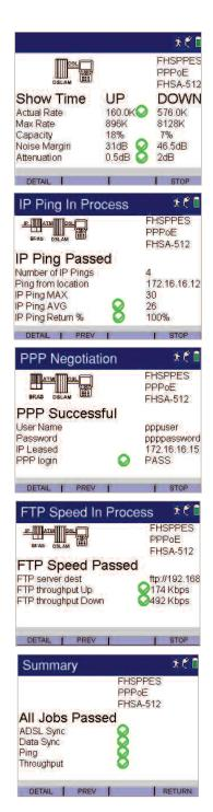
HST-3000 automation features and test scripts display simple pass/fail results that increase technician efficiency and accuracy.
